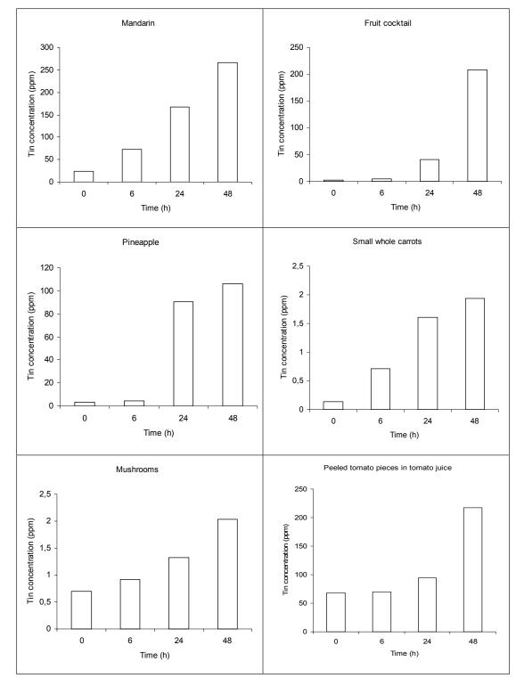
Fig. 1. Effects of standing in an opened can (at 20°C) on tin content in syrup.
